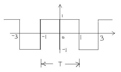
c. Find the trigonometric Fourier series for the periodic signal x(t) in Figure.
