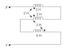
(ii) Derive the expression for coefficient of coupling in terms of mutual and self (8) inductance of the coils.
