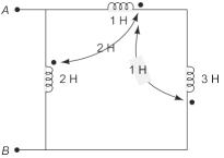
5.(i) Calculate the effective inductance of the circuit shown in Fig. Across XY. (8)
