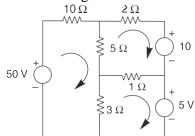
(ii) Determine the voltage at each node of the circuit shown in Fig
