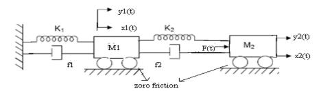
3. Draw the voltage and current analogs for the following mechanical system.
