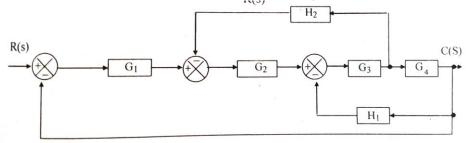
**9.** Find the overall gain C(s) / R(s) for the signal flow graph shown in figure.
