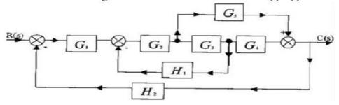
8. Determine the overall transfer function C(s) / R(s) for the system.
