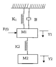
2. Determine the transfer function of the mechanical system shown in figure. Also draw its F-V analogy circuit and F-I analogy circuit.
