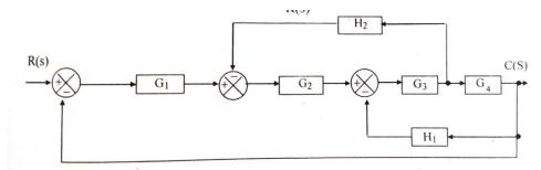
9. Find the overall gain C(s) / R(s) for the signal flow graph shown in figure.
