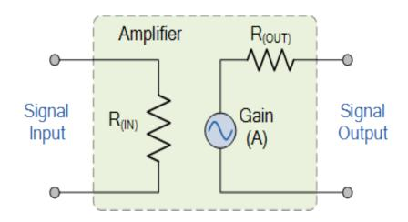
• Amplifier gain is simply the ratio of the output divided-by the input. Gain has no units as its a ratio, but in Electronics it is commonly given the symbol "A", for Amplification. Then the gain of an amplifier is simply calculated as the "output signal divided by the input signal".
