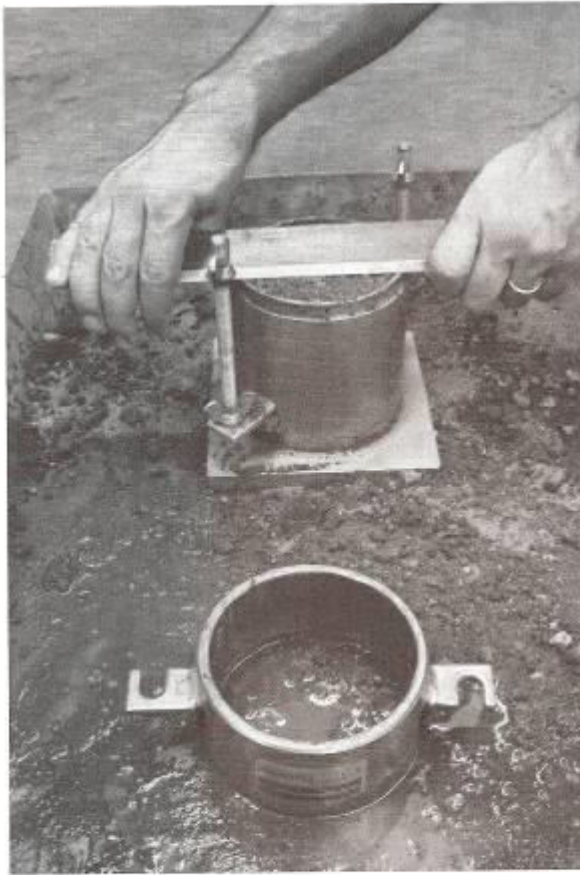
Figure 12.4. Excess soil being trimmed (Step 8).
