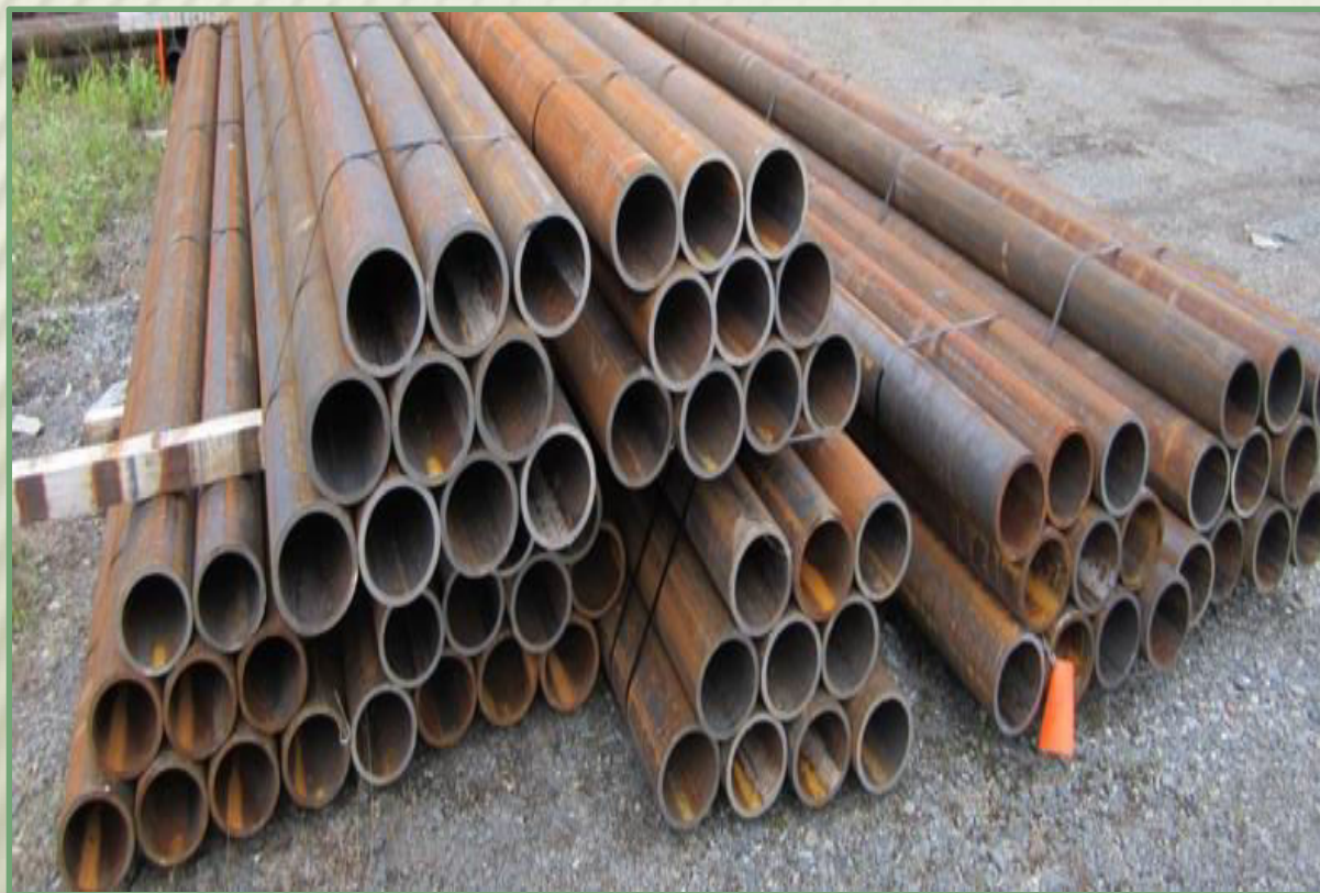
PIPE STEEL PILES
