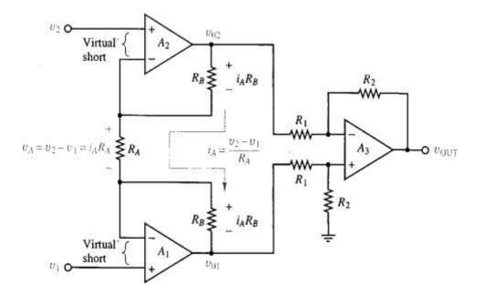
$v_{OUT} = (R2/R1)(1 + [2R_B/R_A])(v1 - v2)$
