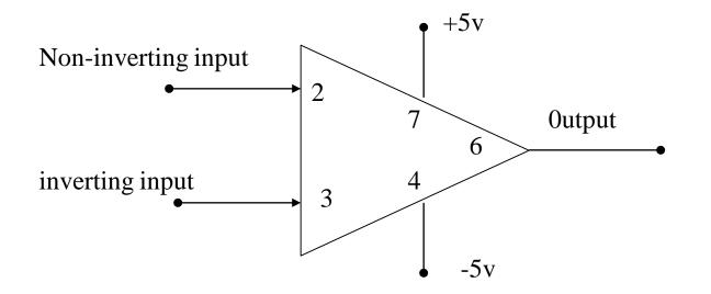
Linear Integrated Circuits – An analog IC is said to be Linear, if there exists a linear relation between its voltage and current. IC 741, an 8-pin Dual In-line Package (DIP)op-amp, is an example of Linear IC.
