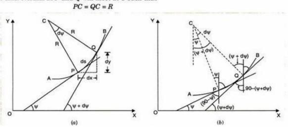
The point C is known as centre of curvature of the curve PQ.
