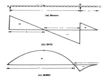
1. Draw the SFD and BMD for the beam which is loaded as shown in the fig. Determine the point of contraflexure within the span AB.
