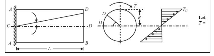
Maximum twisting torque or twisting moment
