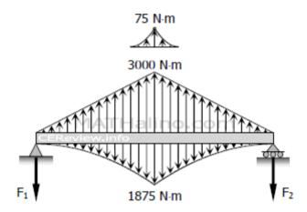
Conjugate Beam Loaded with M/EI Diagram
