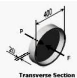
(b) From (a),  $\sigma_t = \frac{pD}{2t}$  and  $\sigma_l = \frac{pD}{4t}$  thus,  $\sigma_t = 2\sigma_l$ , this shows that tangential stress is the critical.
