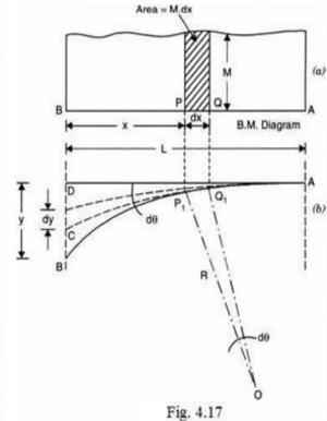
Slope And Deflection Of Simply Supported Beam Carrying A Point Load At The Centre By Mohr's Theorem
