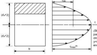
(Shear stress is distributed parabolically over a rectangular cross-section, it is maximum at y=0 and is zero at the extreme ends)
