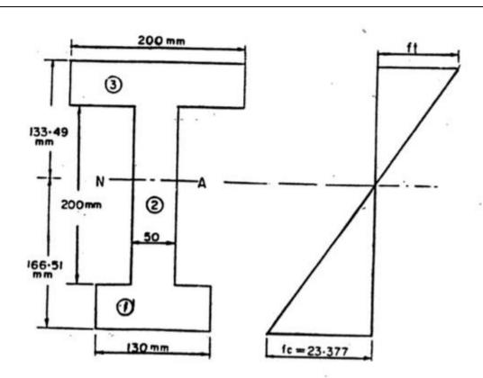
This stress will be compressive. In case of cantileers , upper layer is subjected to tensile stress, whereas the lower layer is subjected to compressive stress.
