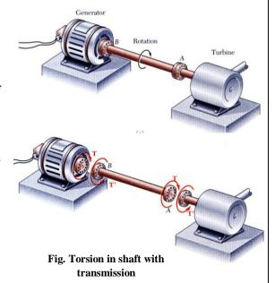
The shafts are designed on the basis of strength and rigidity.
