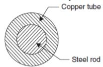
**Solution:** Area of steel rod  $A_s = \frac{\pi}{4} \times 25^2 = 490.87 \text{ mm}^2$
