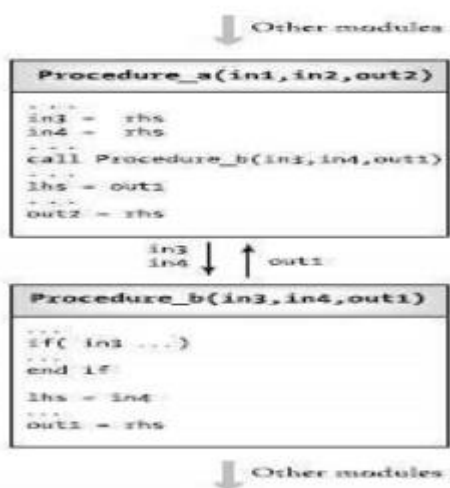
Fig. 6.9 Example integration of two procedures.
