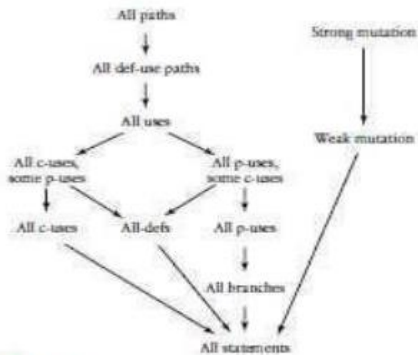
FIG. 5.5 A partial ordering for test adequacy criteria.
