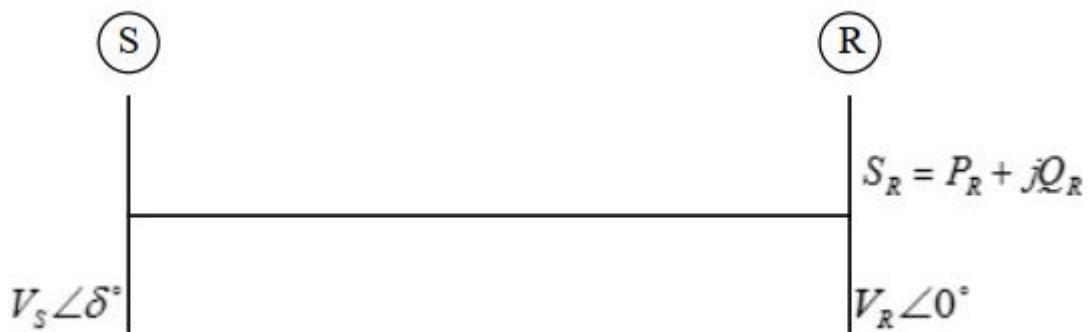
FIG.-. TRANSMISSION LINE POWER FLOW
