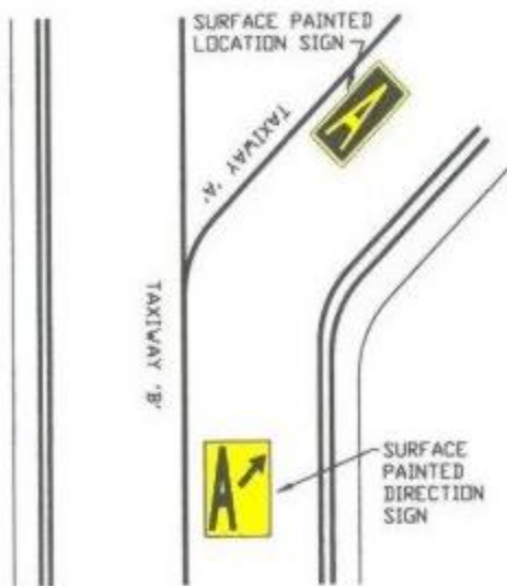
Surface Painted Taxiway Direction Signs
