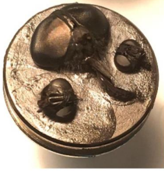
Whole insect heads mounted on a stub and coated with gold
