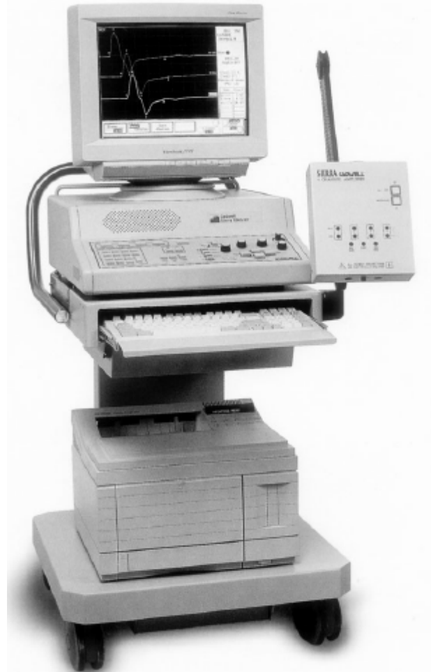
PC based digital EMG recording and reviewing system for 2 to 4 channels
